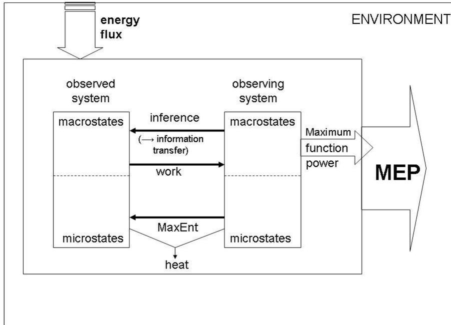
The diagram shows an open system that is embedded into the environment, and which is turn consisting of two systems which stand in the causal relation of observation with each other. This is the most simple form of a hierarchical structure. The observing system manifests a function with reference to the higher-level system, such as an adaptation in an ecosystem. Then, the conjoint hypotheses of MaxEnt and MEP imply:
